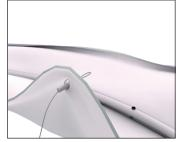
6.Thread cable support through eyelet.
